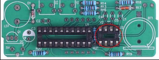
Step 9: Install 2pcs 5pF Ceramic Capacitor at C4,C5.
