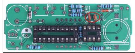
Step 10: Install 2pcs 0.1uF 104 Ceramic Capacitor at C1,C2.
